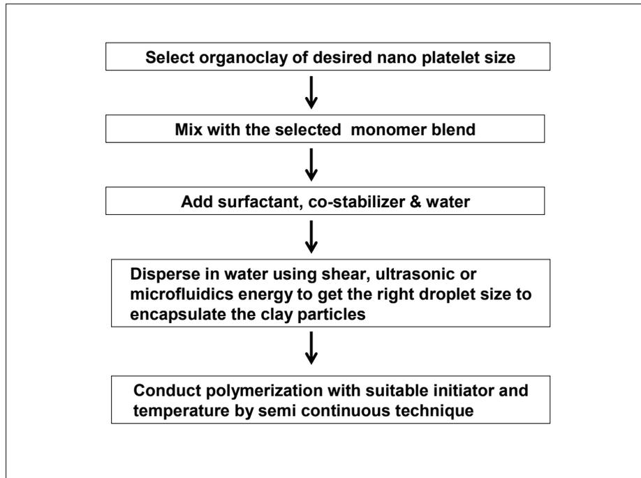
Fig 2: Encapsulation by miniemulsion polymerization.
