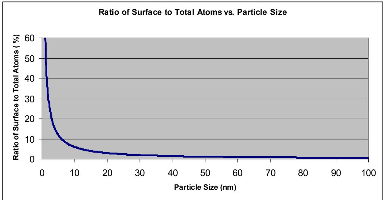
Figure: Surface to Total Atoms expressed as % against Particle Size in nm
