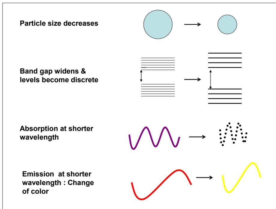
Figure: Change of color with particle size in quantum dots
