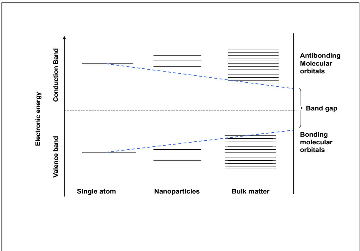
Figure: Band gap change in nanoparticles
