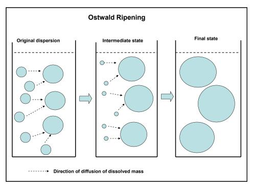
Figure: Ostwald ripening leading to coarse particles on keeping
